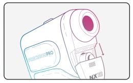
Open the battery door by sliding the panel away from the eye piece.
