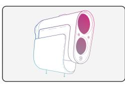
**REMOVE SIDE PLATE:** Pull down on the side plate to remove it from your NX10 rangefinder.
