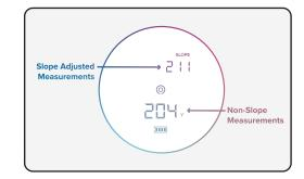
If slope is on, the slope-adjusted number will appear above the aiming circle. The non-slope number will appear below the aiming circle. HOW TO USE
