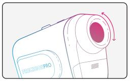
Rotate the dial left or right on the adjustable eyepiece until the display appears sharply focused.
