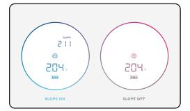
When slope is on, the slope-adjusted distance will appear above the aiming circle. When slope is turned off, the second display will not be shown.
