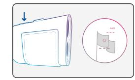
Point the aiming circle at the target -- flag, tree, bunker, etc. Then press and release the POWER button to "shoot your target."
