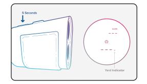
Make sure the screen is off, then press and hold the POWER button for five seconds to change between yards and meters. You will see a Y in the bottom right-hand corner for Yards and a M for Meters.
