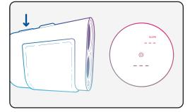
Look through the eyepiece and press the power button to turn on the rangefinder. The aiming circle will appear in the middle of the screen.
