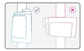
2. When attaching to a frame of a golf cart, make sure that the rangefinder is parallel with the bar. Not perpendicular.
