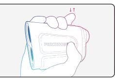
**PRESS AND RELEASE:** When measuring distances, it's important to press and then release the power button.
