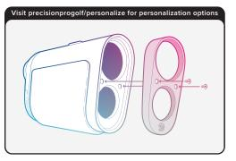
**INSTALLING NEW FRONT PLATE:** Attach new front plate and insert screws. Using the wrench, turn the screws clockwise to fasten the front plate into place.
