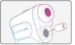
Remove the old battery and insert the new battery to match the image shown above.
