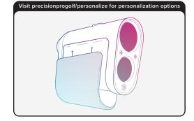
INSTALLING NEW SIDE PLATE: Slide the new side plate up into the grooves of the NX10
